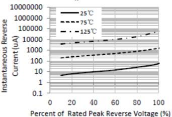
Figure 4. Typical Reverse Characteristics
