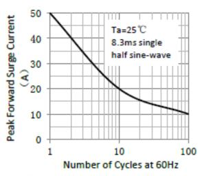
Figure 2.Maximum Non-Repetitive Peak Forward Surge Current
