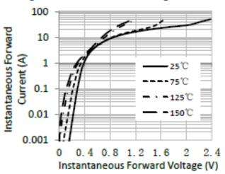
Figure 3. Typical Instantaneous Forward Characteristics
