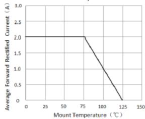
Figure 1.Forward Current Derating Curve
