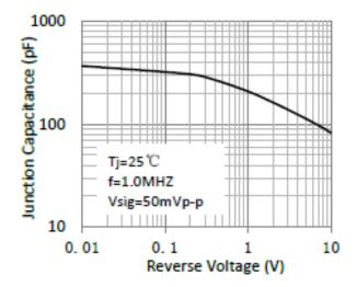
Figure 5. Typical Junction Capacitance
