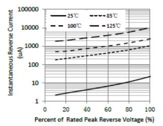
Figure 3. Typical Reverse Characteristics
