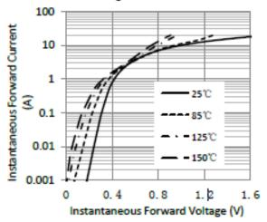
Figure 4. Typical Instantaneous Forward Characteristics
