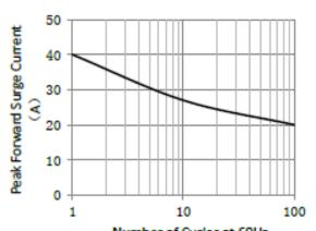
Number of Cycles at 60Hz Figure 2.Maximum Non-Repetitive Peak Forward Surge Current
