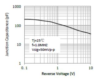
Figure 5. Typical Junction Capacitance
