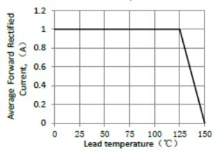
Figure 1.Forward Current Derating Curve
