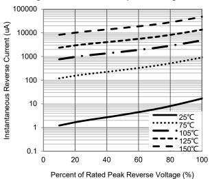
Fig.4 - Typical Reverse Current Characteristics
