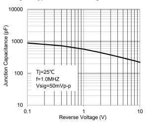
Fig.5 - Typical Junction Capacitance
