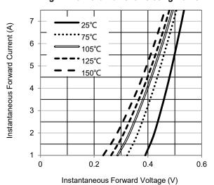
Fig.3 - Typical Forward Voltage Characteristics
