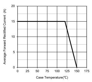
Fig.1 - Forward Current Derating Curve
