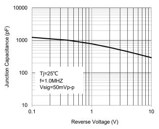
Fig.5 – Typical Junction Capacitance
