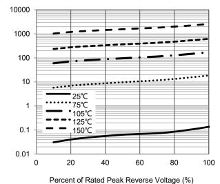
Fig.4 – Typical Reverse Current Characteristics
