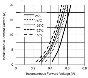
Fig.3 - Typical Forward Voltage Characteristics
