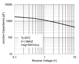
Fig.5 - Typical Junction Capacitance
