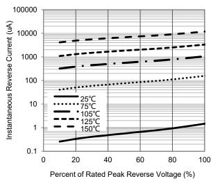
Fig.4 - Typical Reverse Current Characteristics
